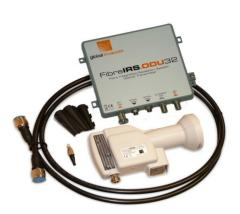
Fully weatherproof, the ODU32 is designed for mounting at the antenna location. It accepts and combines signals from the Wholeband LNB and digital terrestrial antennae (DTT/DAB/FM) which then modulates a laser inside the ODU32. Two optical outputs (FC/PC) are provided for distribution through a Passive Optical Network (PON) of FibreIRS Optical Splitters. Each output of the ODU32 can feed a PON of 32 points or with reduced splits support a reach of 10km.
